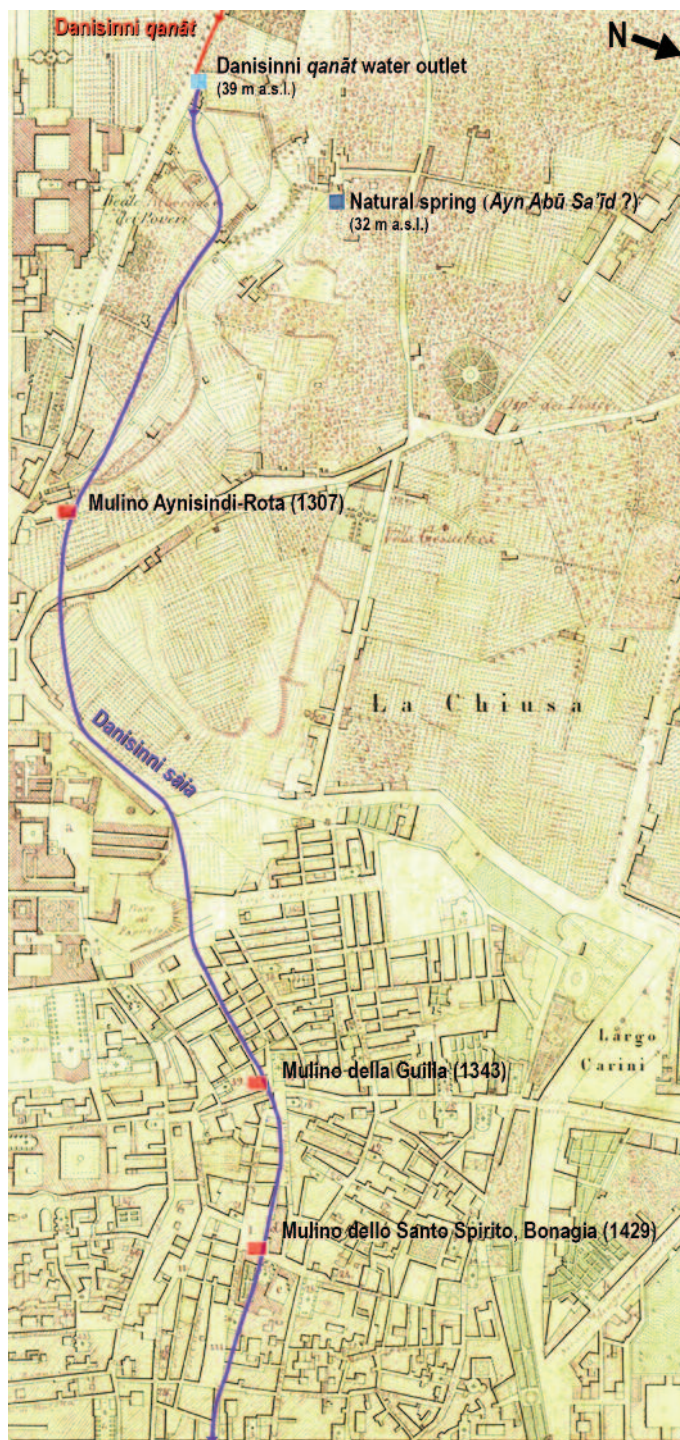
Fig. 9. Danisinni water system: the natural spring along the Papireto river, hypothetically the medieval Ayn Abū Saʿīd (dark blue square); the path of Danisinni qanāt (red line) and its related water outlet (blue square); reconstruction of the canal ( sàia ) (blue line), masonry no longer existing today whose presence was derived from the hill's contour lines, which provided water energy to medieval mills (red squares) in the Papireto valley (Base map: topographic map, scale 1:5000, of Italian Military Geographic Institute, 1863; cartella n. 88, inv. n. 9028 documento n. 17 CRICD-Palermo).
