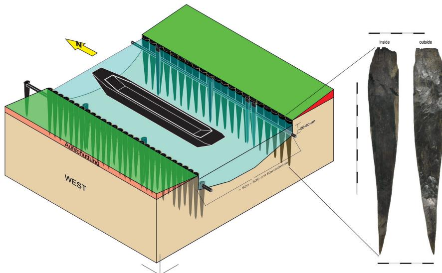
Fig. 9. Reconstruction of the canal construction of the *Fossa Carolina* dated to 793 AD based on the excavation 2013 with an original oak pile of the bank reinforcement (drawing F. Herzig, L. Werther).
