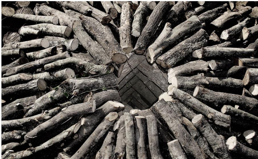
Fig. 5. Chimney of a current charcoal kiln in Croceferrata (Serra San Bruno - Vibo Valentia, Italy - 2007).
